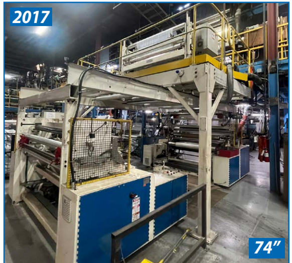
PARTIAL VIEW OF ALPHA MARATHON SURFACE WINDERS AND SECONDARY NIP W/ SLITTING STATION
